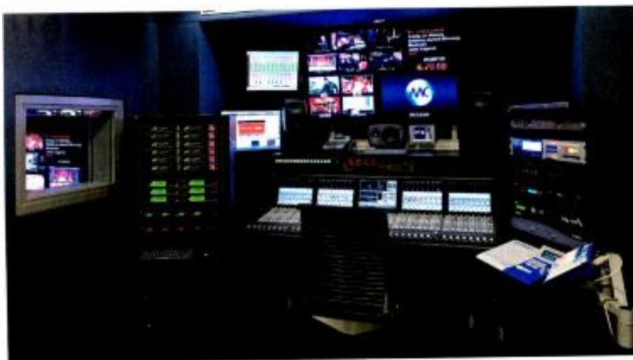
Adjacent to the control room is the audio mixing suite. The overall communications system is based on a Riedel 136 x 136 matrix with a combination of analog, MADI, and AES and GPI interface cards.
