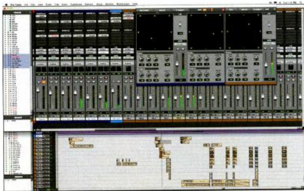
The Avid Pro Tools 10 panner provides a separate LFE fader, which allows for more control. If not managed correctly, however, it may result in too much LFE information being sent to a home system's subwoofer, which can cause the audio to sound "muddy."
